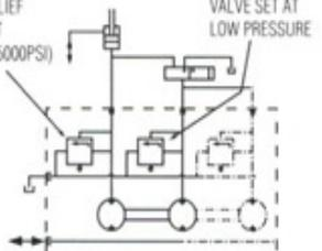
Rotary Flow Dividers split the input flow from a single supply into 2 or more outputs of equal or unequal flows.
