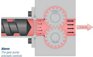
The gear pump precisely controls the amount of polymer flowing from the extruder and removes any pulsation in the flow
